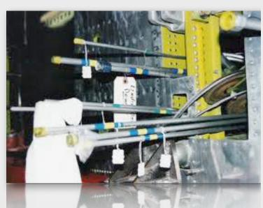
how simple this component is, it requires a specific "torque" to keep it reliable in maintaining plumbing system integrity. You may have seen a maintenance record entry where the sign-off stated, "Tightened B nut." Does this mean it was tightened enough to stop a leak, or was it tightened to a specific torque? If you are just tightening the "B" nut, you could be setting the stage for future failure or fracture.
